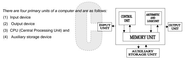
The block diagram shows the primary units or components of a computer.
